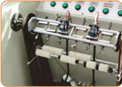
Wire bending test
