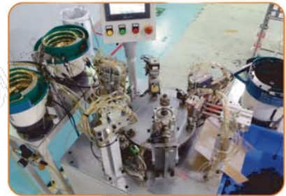
Automated connector production equipment
